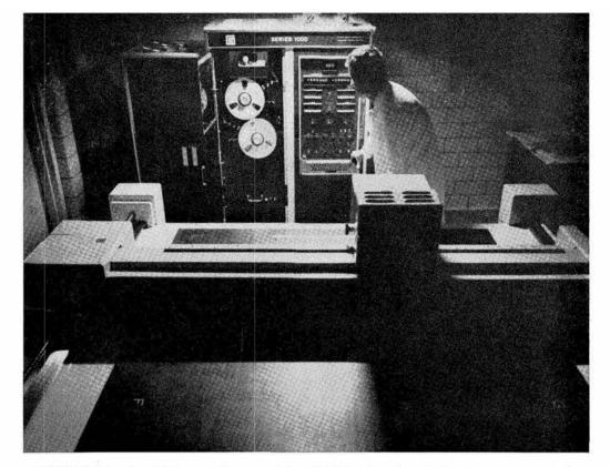
EIGHT-FOOT auto-drafting machine, precision light head and control system are operated by Ronald G. Cheek. Unexposed film is positioned on plotting board, the computer program directs the light head to create the circuit drawing on film. The system is faster than the old manual methods, and a more precise product results.
